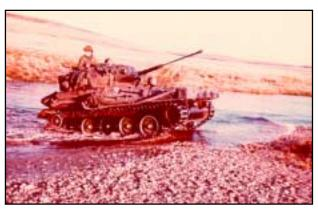
Photo at left of a Chinook cargo helicopter hovering over two British armored vehicles gives some sense of the barren landscape, devoid of cover. Above, a lightweight Scimitar (only 8 tons) moves easily over the boggy terrain.
