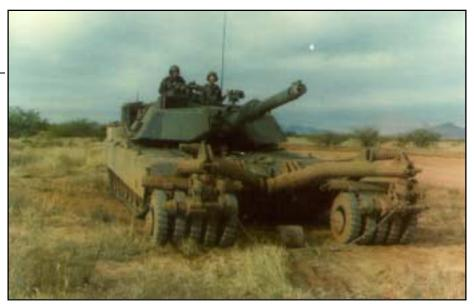
Mine rollers are the best method to find the edge of a minefield and the best way to proof a breach lane, according to the author.
