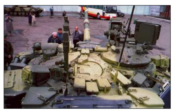
The view from the top of the turret of a T-90 is impressive for the sheer number of hatches, boxes and accessories that clutter the turret roof, much of it related to the tank's self-protection system.
