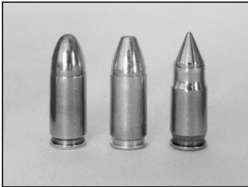
**Penetration capability of current service pistols could be greatly increased by switching from standard 9mm ball ammo (left) to a hard-core, very high-velocity 9mm round (center), or a “necked-down” cartridge with reduced-diameter, lightweight bullet (right). Use of the latter would necessitate a barrel change, but should be compatible with 9mm magazines if the cartridge case is properly designed.**
