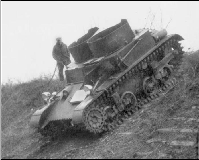
Above, the Ordnance-sponsored T5 Combat Car descends a slope during testing. Its vertical volute spring suspension was later a common feature of U.S. light and medium tanks, but the idea of twin turrets was abandoned for tactical reasons.
