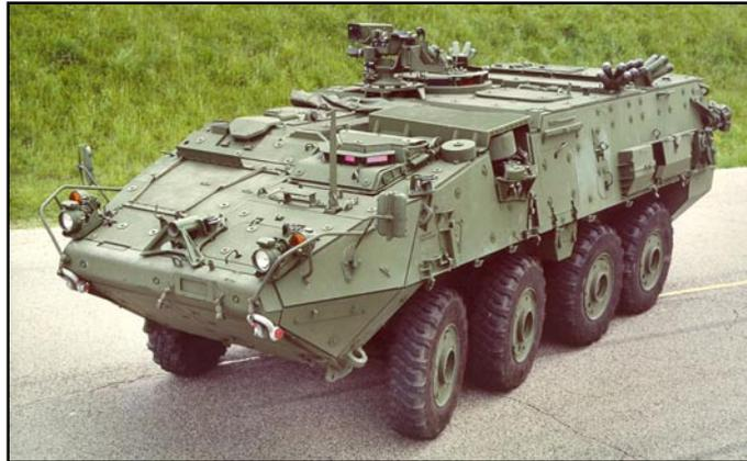
The standard appliqué armor on the LAV III does not protect against hand-held antiarmor weapons like the RPG-7 — the primary threat in urban combat. The author argues for additional protection from kits that would withstand attack from RPG-type HEAT warheads (Photo: GM Defense)
