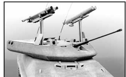
Below, the turret detail shows the pair of missile launchers in the raised position. One launcher is for anti-aircraft missiles, the other for antitank missiles, both Russian weapons.
