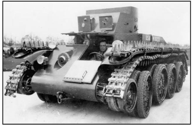
Above, the unusual Christie convertible wheel/track suspension is seen in the wheeled configuration with its tracks stowed above and below the fenders on each side. Called “combat cars” (the cavalry was prohibited from owning “tanks”), the T4 was armed with machine guns.
