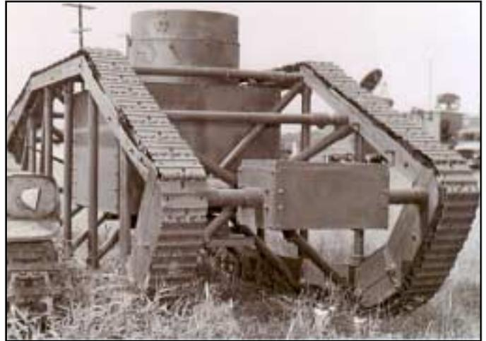
**Wheelock's unusual design kept weight down (9 tons) while retaining cross-country and trench-crossing capabilities. In addition, there was little for the enemy to shoot at. The pipe construction would allow the tank to be dismantled and shipped, then reassembled on arrival in theater. The two-man crew rode in the half-inch-thick armored box suspended from the frame.**
