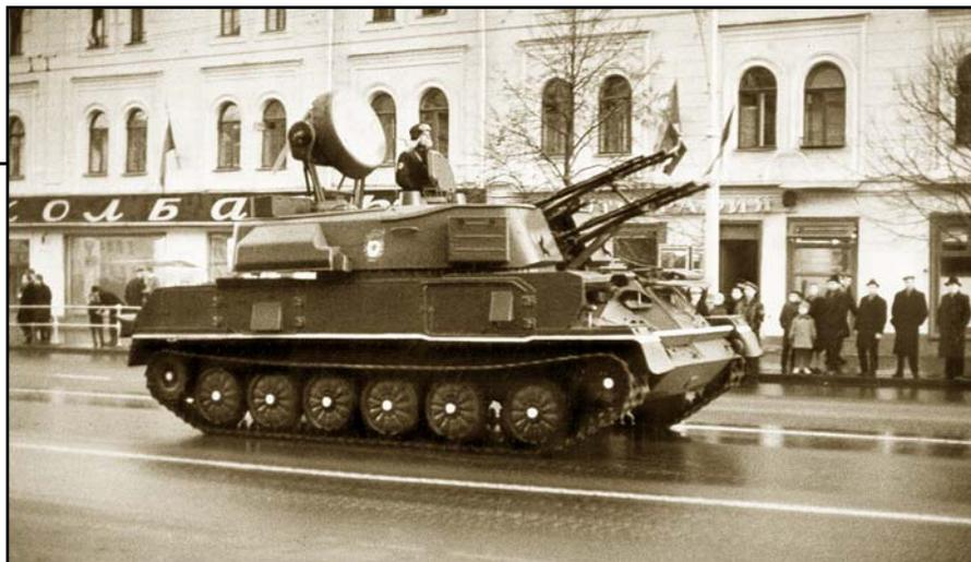
The Soviets employed the ZSU-23 air defense weapon against guerrillas perched high along mountain passes because the four 23mm machine guns, designed to hit planes, could elevate sufficiently where tank guns could not. Recently, this weapon was also found useful in engaging snipers in tall buildings in Chechnya.
