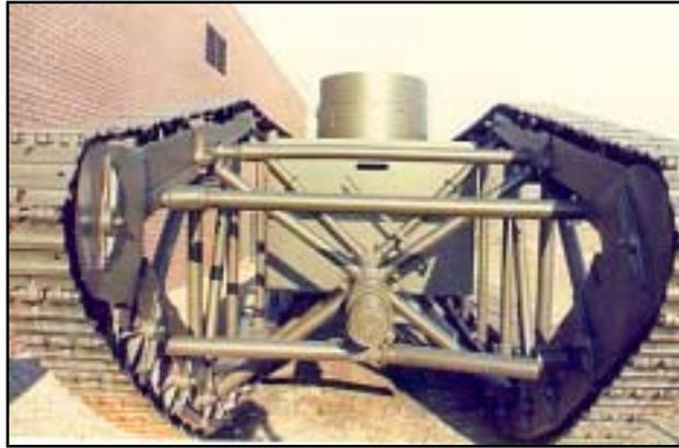
**Wheelock's Skeleton Tank was constructed of standard threaded pipe sections. Only the fighting compartment was armored. This design may have preceded the British concept made famous during World War I.**
