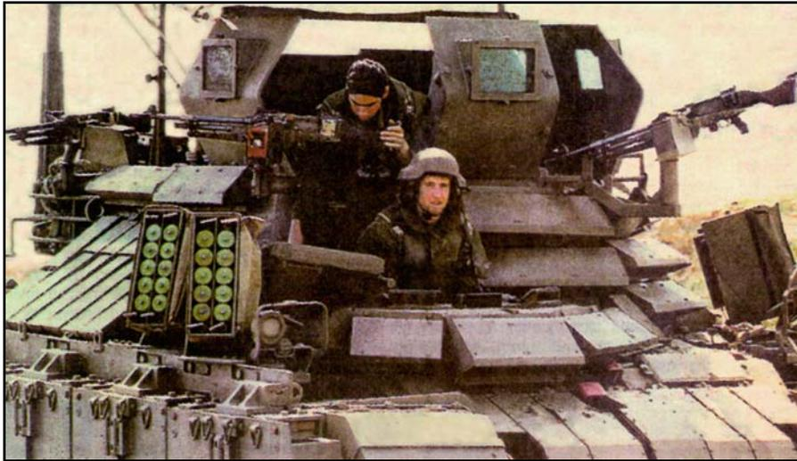
**Note the extent of modifications to this Israeli M113, which is hardly recognizable as such. An armored turret, extra machine guns, reactive armor, anti-RPG plates, and a battery of smoke grenade launchers were added for protection against guerrillas, but ultimately, even these changes proved inadequate, leading to the modification of obsolete tanks as a more survivable solution.**
