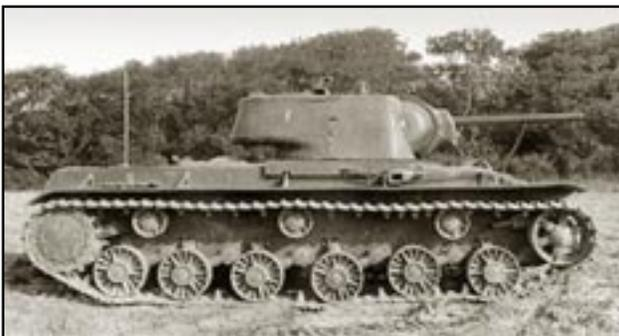
This KV-1 Model 1941, has a cast turret and main gun similar to the F-34 gun of the T-34/76 tank. Mechanical failures took more of a toll than the enemy, and many were abandoned due to lack of repair time.
