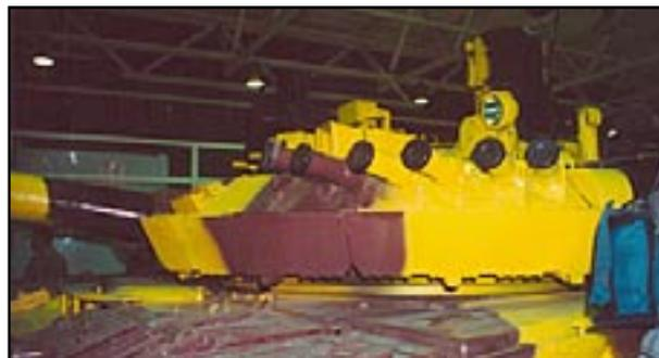
At left, the arrow indicates the digital box in a T-80U (improved) commander's station; above, a T-80UM1 (improved) turret with ARENA-E active protection system.
