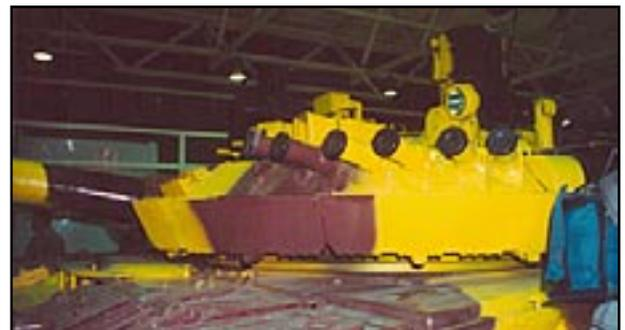
At left, the arrow indicates the digital box in a T-80U (improved) commander's station; above, a T-80UM1 (improved) turret with ARENA-E active protection system.
