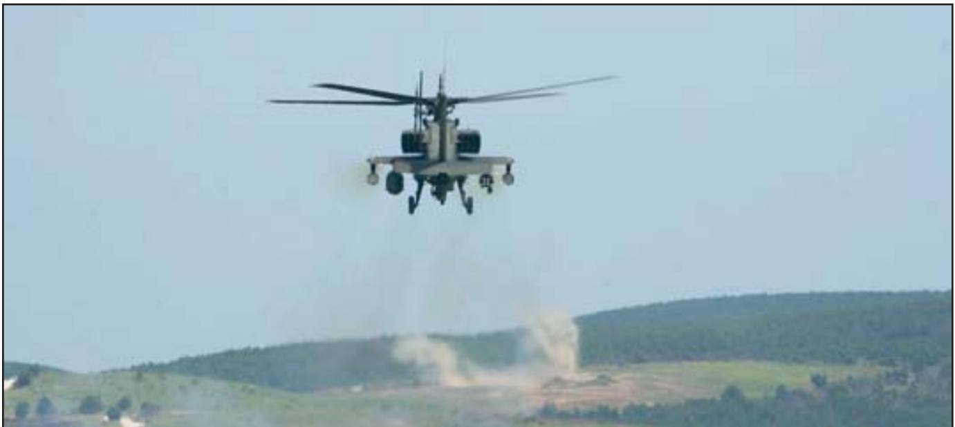
“The M230E1 30mm chain gun is the attack aviator’s preferred implement for cutting the heart out of an insurgency. With a rate of fire of 650 rounds per minute, the cannon sprays high-explosive dual-purpose projectiles with a lethal bursting radius of 4 meters. While the maximum range of the gun is 4,200 meters, engagements are most often made with the IHADSS at ranges of less than 1,000 meters in Iraq. Maximum capacity is 1,200 rounds of 30mm ammunition. The cannon is devastatingly effective against dismounted personnel and soft-skinned vehicles.”
