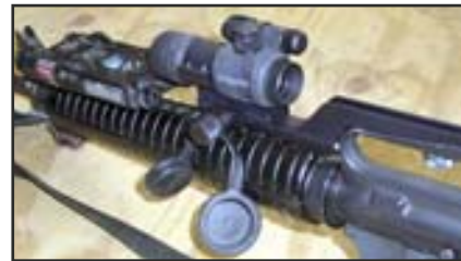
Above and right, an M68 close combat optic mounted in conjunction with the AN/PEQ-2A aiming light on an M16A2. Note that the M68 mounting bracket cannot be mounted to the top carrying handle of the M4 or M16A4.
