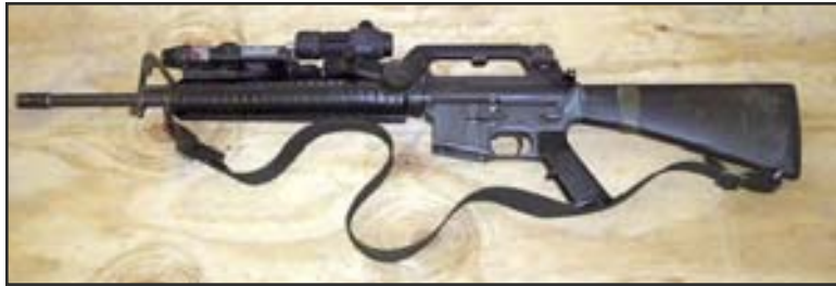
Above and right, an M68 close combat optic mounted in conjunction with the AN/PEQ-2A aiming light on an M16A2. Note that the M68 mounting bracket cannot be mounted to the top carrying handle of the M4 or M16A4.
