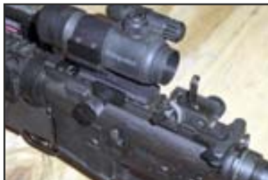
The M4 MWS above mounts the AN/PEQ-2A on the right side since the upper rail of the handguard is taken up by the grenade launcher's leaf sight. Note the BIS is flipped up.
