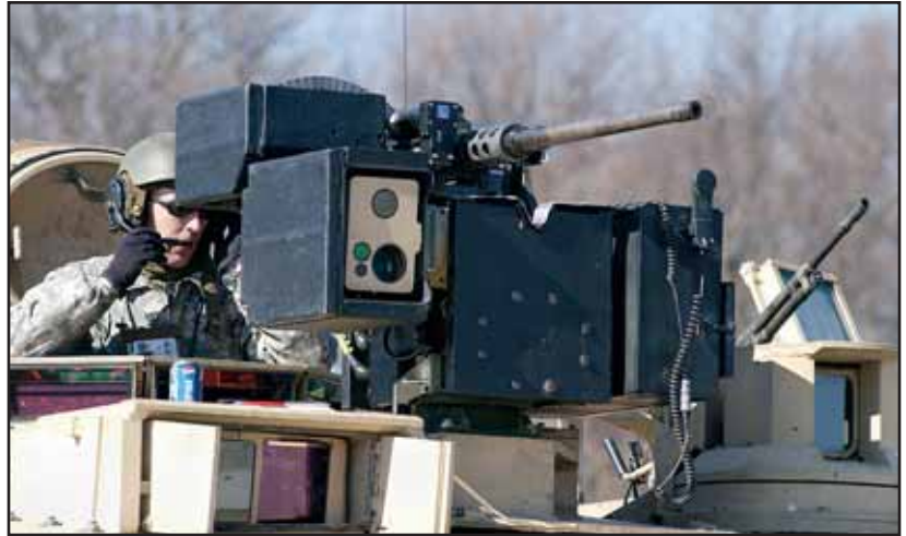
At left, the M240 gun mount; above, the common remotely operated weapons station (CROWS); below left, the tank infantry phone (TIP); and below right, the loader's armored gun shield (LAGS) with light weapon thermal sight (LWTS).
