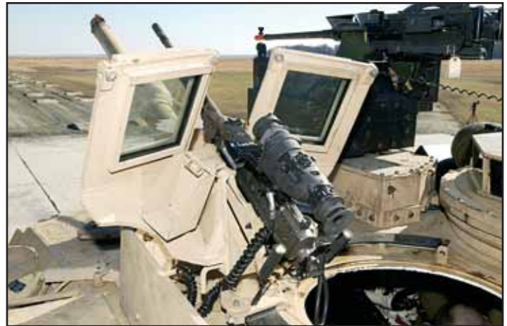
At left, the M240 gun mount; above, the common remotely operated weapons station (CROWS); below left, the tank infantry phone (TIP); and below right, the loader's armored gun shield (LAGS) with light weapon thermal sight (LWTS).
