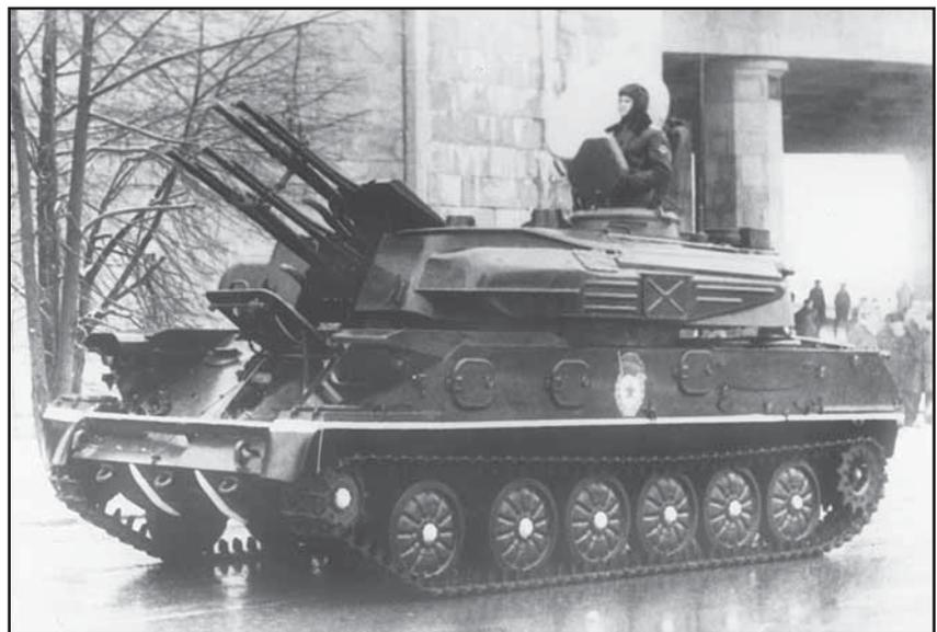
*"The Russians discovered that the thinly armored ZSU 23-4 self-propelled antiaircraft gun was the optimum system for tank support in city fighting, but its vulnerability offset the efficiency of its four 23mm automatic cannons. To ensure the survivability of tanks, they needed a new system that was built like a tank, but provided mutual close combat support."*
