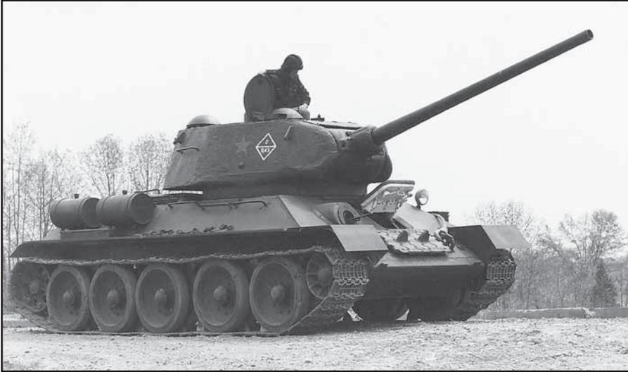
*"The main Soviet tanks of World War II were the T-34-85 medium tank and the KV1 heavy tank. The T-34-85 weighed 32 tons, had a five-man crew, and carried an 85mm cannon and two 7.62mm machine guns. The KV1 weighed 47.5 tons, had a five-man crew, and carried a 76mm cannon and four 7.62mm machine guns."*
