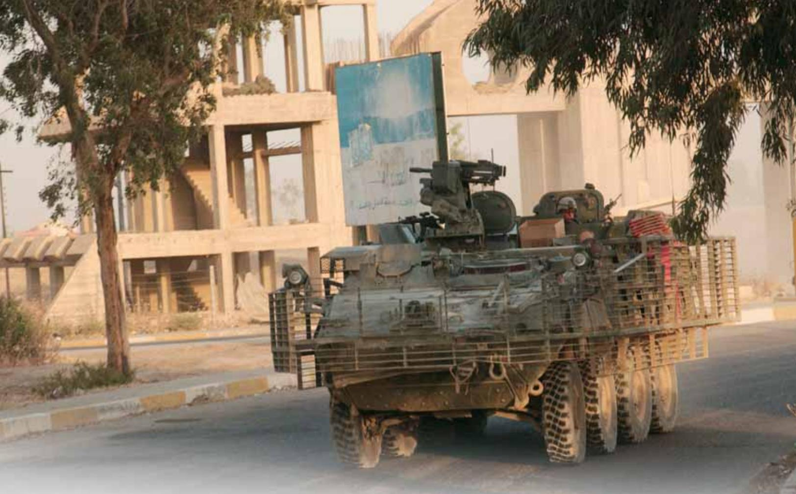
*“The Stryker reconnaissance squadron is unique for two reasons: use of the Stryker vehicle as the standard platform and the addition of an unmanned aerial system (UAS) unit. The Stryker was built with digital integration in mind and connects scouts with the SBCT by digital data, as well as voice.”*
