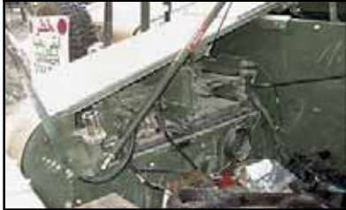
Figure 1. At left, the best location for the CPU and VAA is in the back, on the driver side quarter-panel inside the M1151 right above the wheel well.
