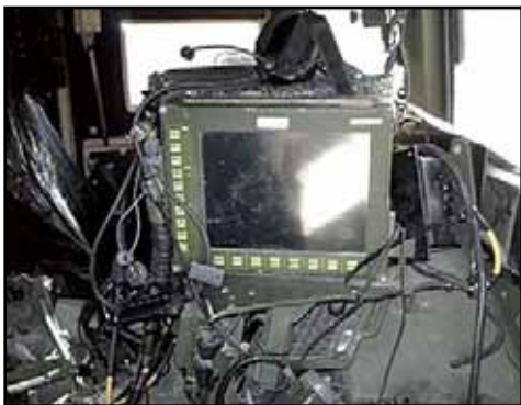
Figure 4. The mount for the AN/UYSK-128 display is installed up front near the passenger side, as well as the mount for the PSN-11 PLGR.
