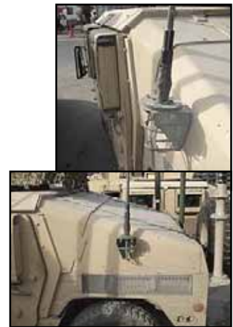
Figure 3. The EPLRS antenna and antenna mount are mounted on the outside driver side right above the rear wheel well.
