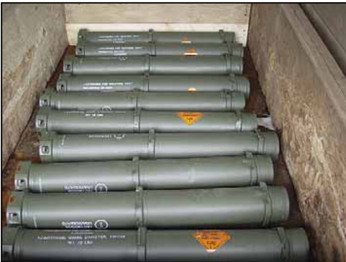
Figure 2. Unconstrained tank rounds undergo loose (unsecured) cargo testing.
