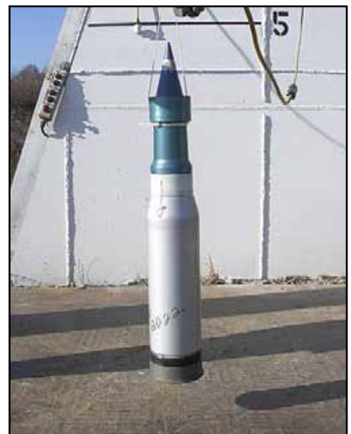
Figure 4. A 120mm tank round undergoes the 1.5-meter bare drop test.
