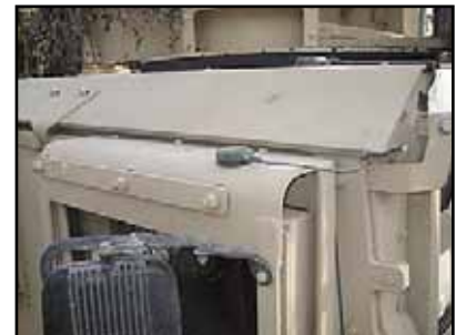
Figure 5. The PSN-11 PLGR antenna can be mounted right above the front passenger side, on the outside of the HMMWV. Most of these are magnetic, or can be secured with Velcro.
