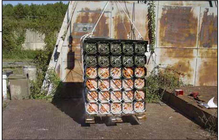
Figure 3. The 2.1-meter drop test is conducted on a sling-loaded pallet.
