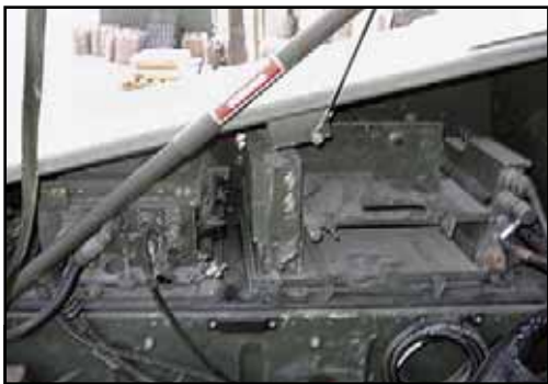
Figure 1. At left, the best location for the CPU and VAA is in the back, on the driver side quarter-panel inside the M1151 right above the wheel well.
