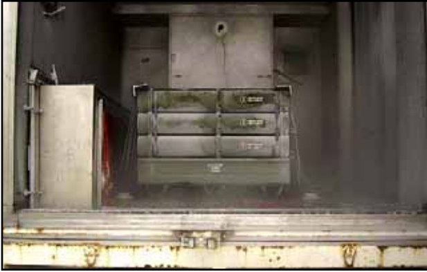
Figure 1. The pallet above has been conditioned to a cold temperature for secured cargo testing. At right, a six-round tank hull ammunition rack undergoes vibration testing.
