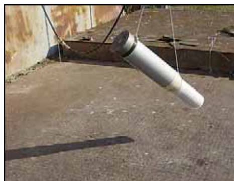
Figure 4. A 120mm tank round undergoes the 1.5-meter bare drop test.
