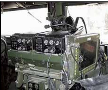
Figure 4. The mount for the AN/UYSK-128 display is installed up front near the passenger side, as well as the mount for the PSN-11 PLGR.
