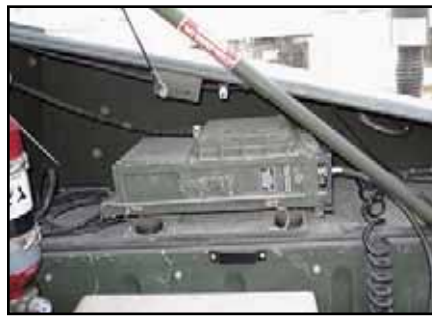
Figure 2. Above, the mount for the EPLRS is installed on the right quarter-panel (passenger side) above the wheel well.
