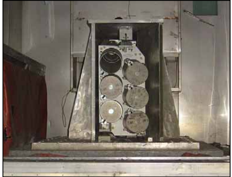
Figure 1. The pallet above has been conditioned to a cold temperature for secured cargo testing. At right, a six-round tank hull ammunition rack undergoes vibration testing.
