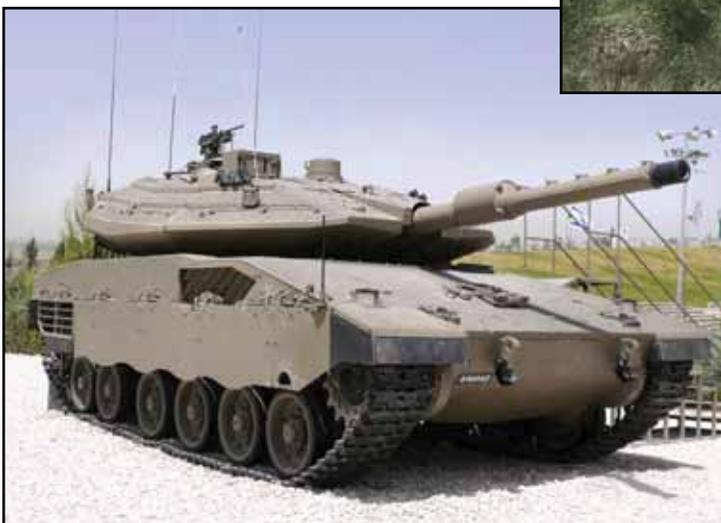
*“Older generation tanks are still highly vulnerable to side, rear, top, or bottom attacks. The multidirectional aspect of the threats in urban areas makes it easier for an attacker to target these weak points. Modern tanks, such as the M1, Leclerc, Challenger, and Merkava have seriously improved their protection with a whole array of highly efficient add-ons, which adapt to the threat and conflict level.”*
