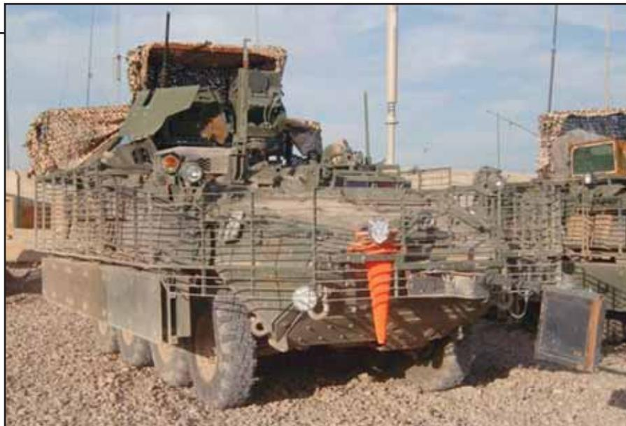
*"An active enemy sniper cripples a gunner's ability to effectively observe his sector. Other common primitive modifications include sandbagging around hatches and securing HMMWV glass to cupolas, often referred as "pope glass." Our recce gunners are making primitive modifications to increase their odds of survival during enemy direct-fire contact."*
