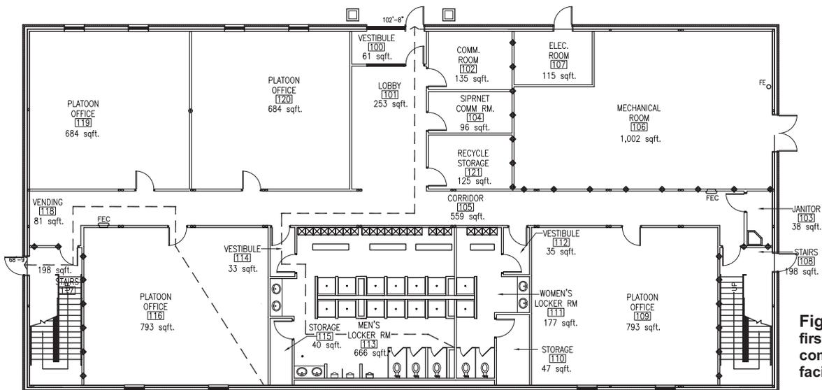
Figure 3. At left, first-floor layout of a company operations facility.
