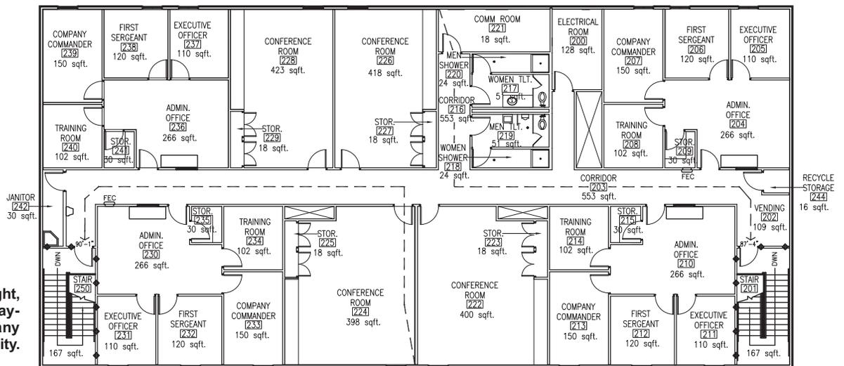
Figure 4. At right, second-floor layout of a company operations facility.
