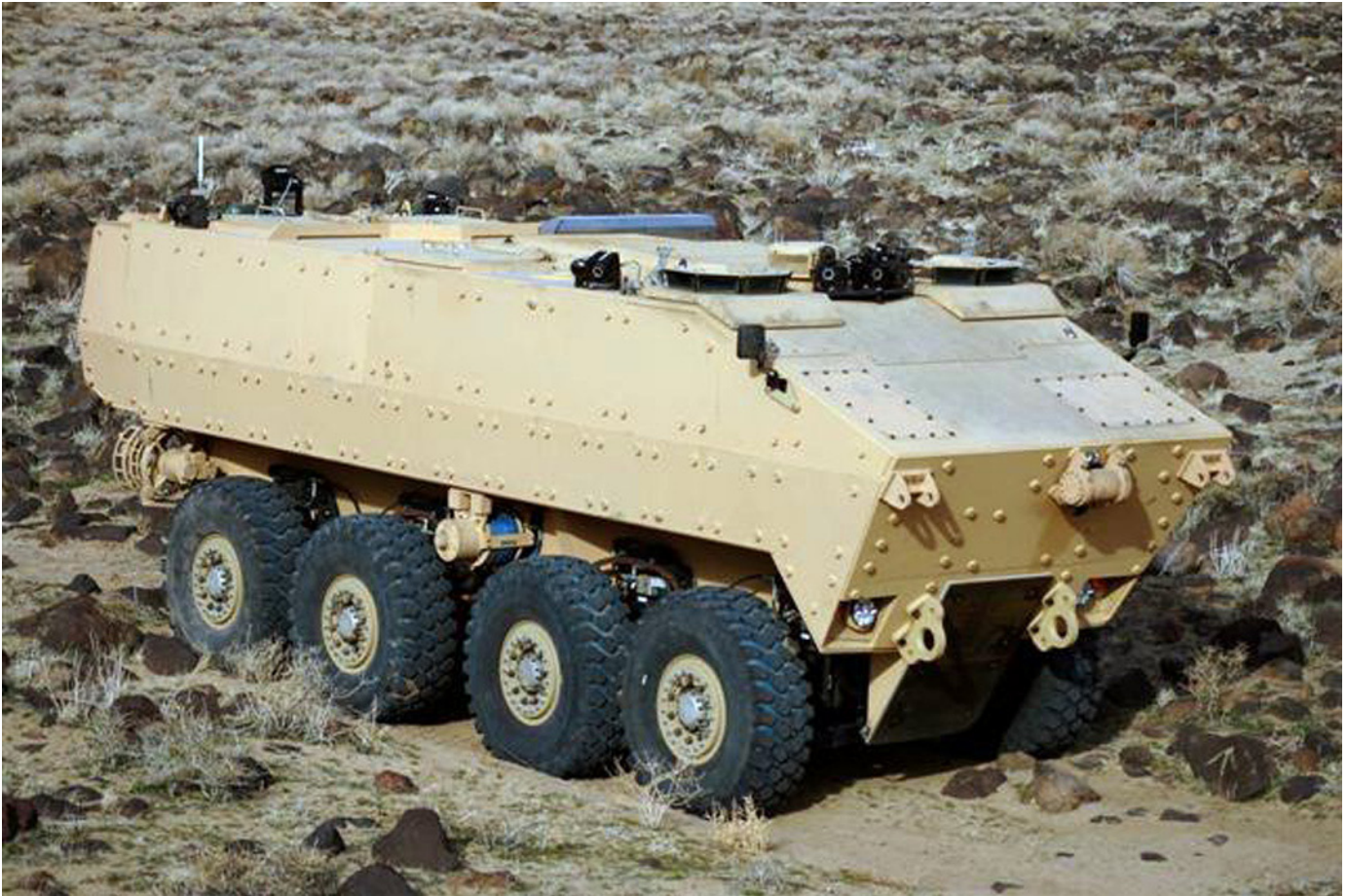
Figure 1. MPC technology demonstrator. The MPC is the first phase of the U.S. Marine Corps' effort to replace its aging Amphibious Assault Vehicle with the ACV. The ACV's mission will be for a pair of them to be able to carry a reinforced infantry squad with two days of supply at speeds compatible with the M1A1.
