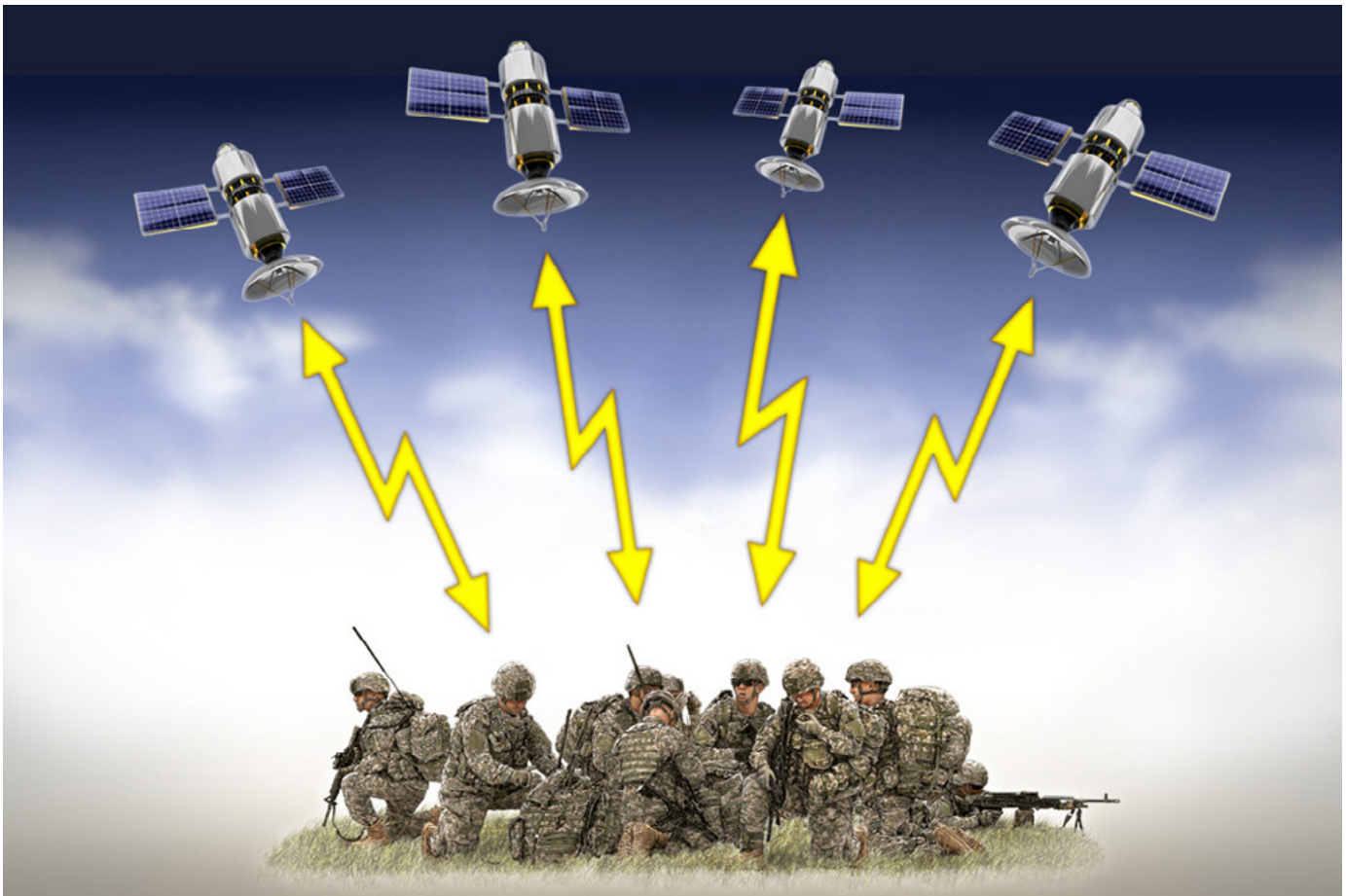
Figure 4. Unfavorable satellite geometry. This graphic depicts satellites with less variance in heights, depths and horizontal distances relative to the Soldiers. These satellites are more compactly arrayed than those in Figure 3, degrading the accuracy of the PNT signal.
