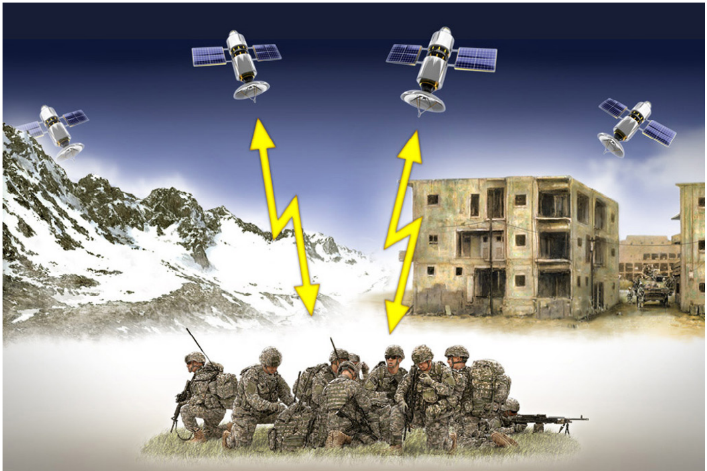
Figure 5. Effects of terrain. Naturally occurring or manmade terrain features can block or reflect GPS signals, reducing the number of satellites in view and preventing your handheld device from receiving the data necessary to get a good geolocation. Leaders should address such potential effects during mission planning.
