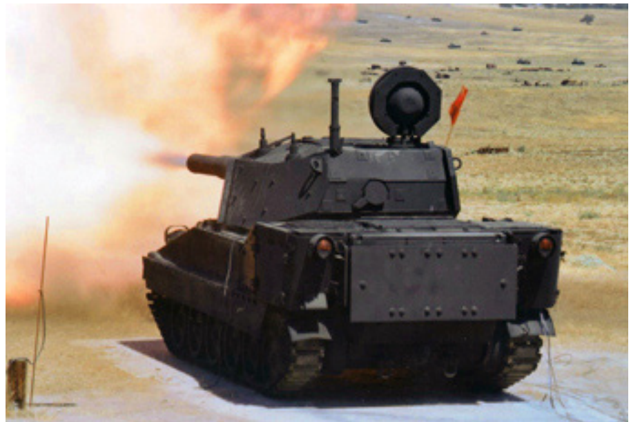
Figure 3. The XM-8 AGS fires its 105mm cannon in a California test.
