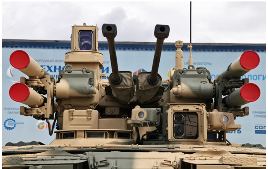
Figure 3. The commander’s panoramic sight (located on the roof) gives the BMPT hunter-killer capabilities by continuously scanning targets for the gunner. (Photo copyright Vitaly Kuzmin, http://vitalykuzmin.net . Licensed under a Creative Commons Attribution-ShareAlike 3.0 Unported License)
