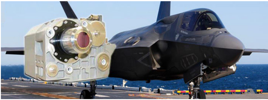
Figure 6. The F-35's DAS allows the pilot to peer through the aircraft body to see high-resolution thermal imagery on a helmet-mounted display as well as automatically detect and classify targets. (U.S. Marine Corps photo)
