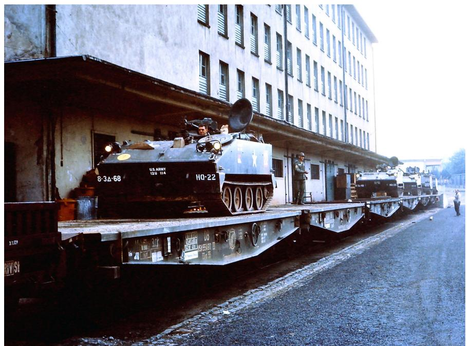
Figure 9. 3<sup>rd</sup> Battalion, 68<sup>th</sup> Armor, conducts rail-loading of M114s in the Baumholder training area, 1965. Rail travel of armored vehicles to major training areas was routine but strictly managed by the Deutsche Bundesbahn.
