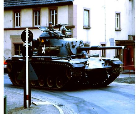
Figure 7. An M60 from 4<sup>th</sup> Tank Battalion, 68<sup>th</sup> Armor, in Germany, 1964, with M2HB on the pintle mount of the commander’s cupola. The M85 machinegun was not issued. The battalion was withdrawn from Germany later in 1964.
