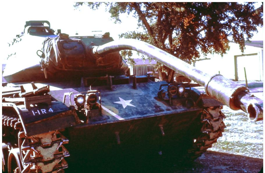
Figure 2. A 1<sup>st</sup> Battalion, 4<sup>th</sup> Cavalry (1<sup>st</sup> Infantry Division), M41 tank at Fort Riley, KS, in September 1963. The photographer's tank ran over its own gun tube when crossing a steep stream bank at night.
