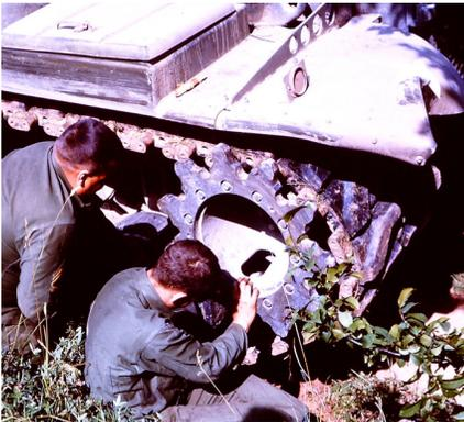
Figure 13, above. Repairing a track thrown to the inside of the sprocket when navigating a narrow path in Germany in 1965. No fun, as the other track was thrown, too.
