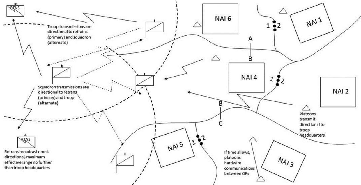
**Figure 3. Example network diagram to reduce electromagnetic signature.**
