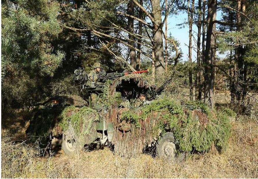
**Figure 1. Netherlands reconnaissance truck camouflaged with natural materials in a concealed position.**
