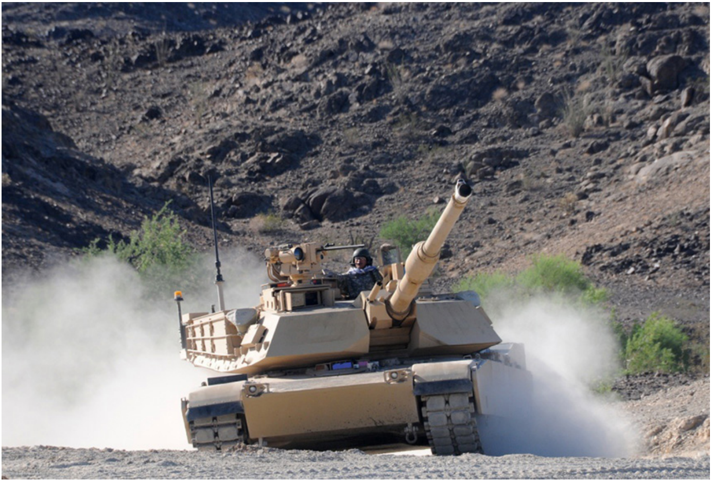
Figure 2. The M1 Abrams is America's sole main battle tank and is considered the best tank in the world. It sports a 120mm main gun and is powered by a 1,500-horsepower turbine engine that makes it highly maneuverable. The M1 has been consistently tested at U.S. Army Yuma Proving Ground, AZ, since its first development in the late 1970s because it is being constantly improved. There are some 8,000 Abrams tanks in the inventory. (Photo by Mark Schauer)
