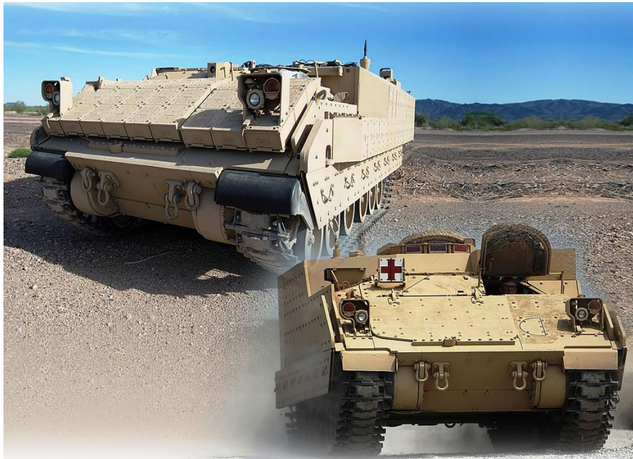
Figure 2. General-purpose and medical-evacuation-vehicle variants of the AMPV.
