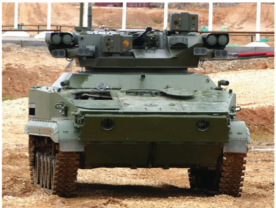
Figure 1. A Russian UGV based on the BMD armored chassis. Russia’s armed forces will likely integrate UGVs with motor rifle battalions because of the Ministry of Defense’s “Weapons Robotizing 2015” program.
