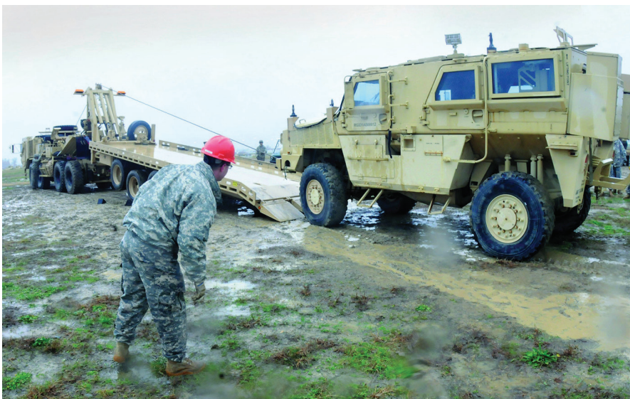
Figure 4. SGT Jeffrey Palmer, an instructor, keeps a careful watch as students in the MCRS module of the H8 Recovery Specialist Course pull a disabled mine-resistant ambush-protected vehicle onto the MCRS' tilt-deck recovery trailer during training at Downer Range, Fort Lee, VA. The H8 course is a three-week additional-skill identifier course at Fort Lee. (U.S. Army photo)
