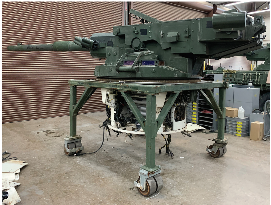
Figure 3. A rewired MGS turret sits on a turret stand in the Longknife Squadron motorpool. (Photo by 1LT John Formica)
