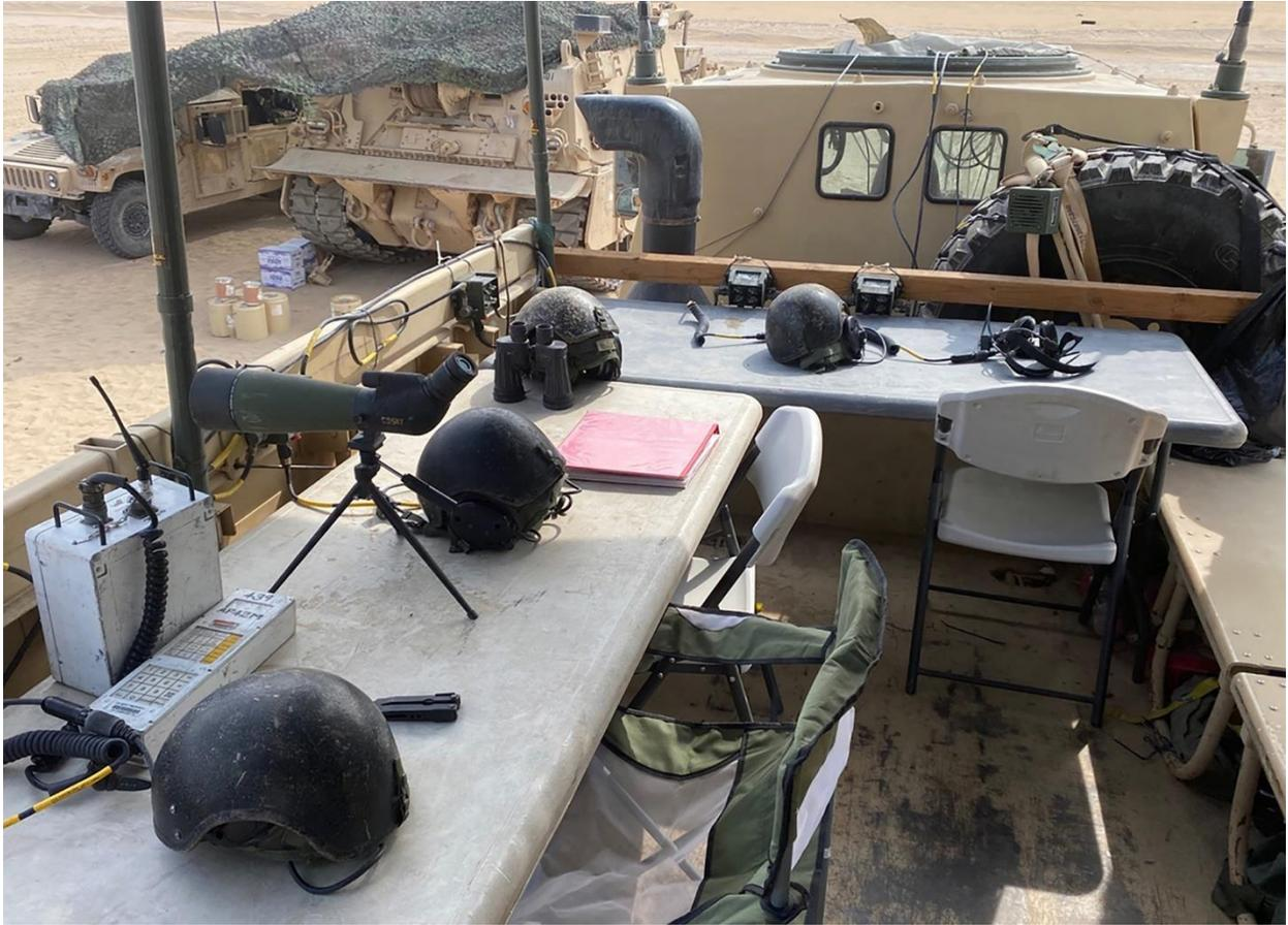
**Figure 3. Target operator station, crew-communication stations and VCE stations setup in the MGT. (Photo by 1LT Jena Ladenburg)**
