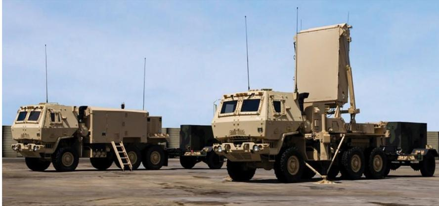
**Figure 4. The AN/TPQ-53 is a C-130-transportable, truck-mounted counter-target-acquisition radar system configured to provide 360-degree threat-detection capability. It is able to locate the firing positions of both rocket and mortar launchers. The Q-53 requires a four- or five-man crew and includes a 60-kilowatt transportable generator and one support-shelter vehicle. Q-53 uses an encrypted wireless network able to reach up to 1,000 meters away. (U.S. Army photo by Kristen Kushiya)**
