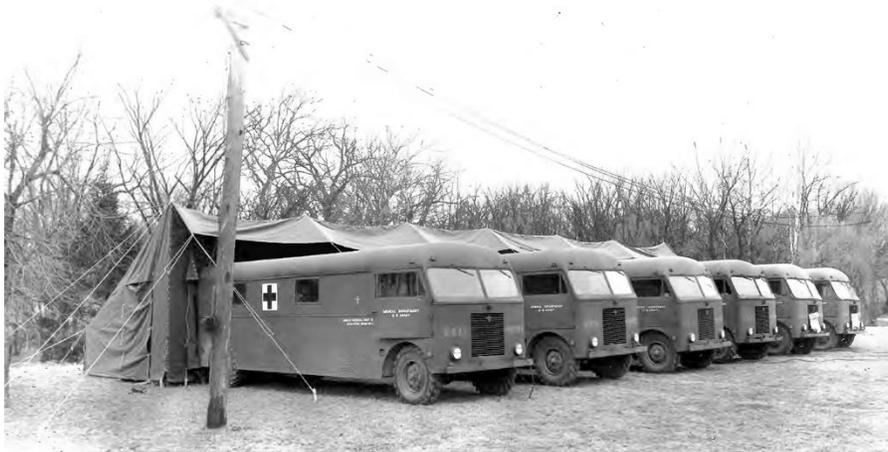
**Figure 4. A mobile surgical unit consisting of trucks with a special operating-room body. During the mid-1930s, MFSS experimented with such vehicles to try to find a solution to providing mobile medical support to mechanized and motorized units. (MFSS scrapbook collection, AMEDD Center of History and Heritage Archives, Fort Sam Houston, TX)**
