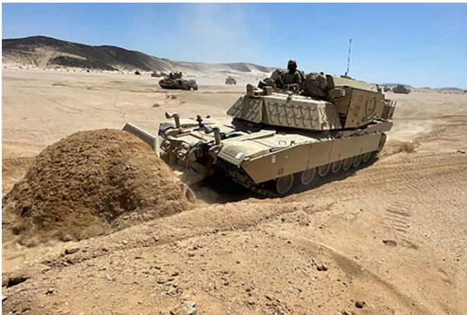
**Figure 4. A 59<sup>th</sup> CEC-A ABV proofs a lane during NTC 22-06 with 2<sup>nd</sup> ABCT, 1<sup>st</sup> Cavalry Division. (U.S. Army photo)**
