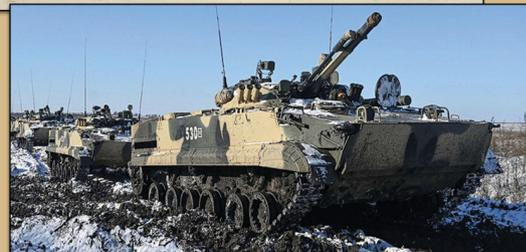
The BMP-3 Infantry Fighting Vehicle has been in service since 1987, successor to the BMP-1 and BMP-2. Features include a stabilized 100mm gun/launcher, able to fire shells or the Bastion ATGM, and a 30mm autocannon. Recent upgrades on some vehicles include a 57mm autocannon and a remote weapons station fitted with (AT-9 Spiral-2) missiles. It can also carry the Shtora-1 electro-optical jammer. In service with numerous countries; Russia being the primary user (720+).
