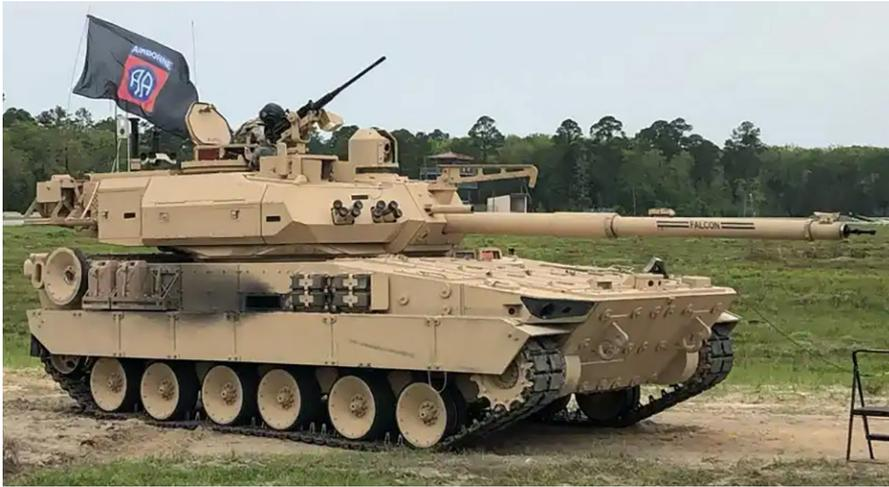
**Figure 3. The MPF ground-combat vehicle from General Dynamics Land Systems. (U.S. Army photo)**
