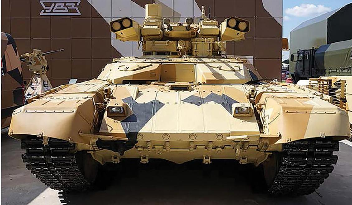
**Figure 7. The latest model of BMPT-72 destined for the export market. Note the redesigned turret and lack of forward-facing grenade launchers. (Photo copyright Vitaly Kuzmin. Licensed under a Creative Commons Attribution-NonCommercial-NoDerivatives 4.0 International License.)**
