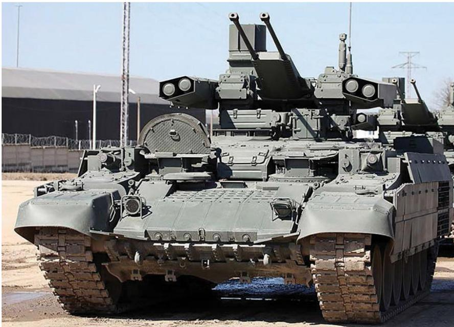
**Figure 1. The Russian army's BMPT-72. The turret has been modified from earlier models, with armor surrounding the ATGM tubes and some other changes, but the hull retains the grenade launchers. (Photo copyright Vitaly Kuzmin. Licensed under a Creative Commons Attribution-NonCommercial- International License NoDerivatives 4.0.)**
