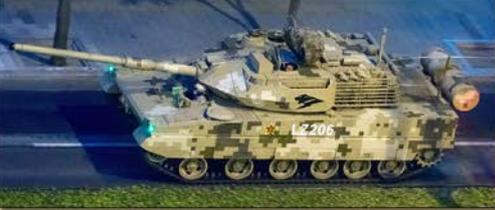
Chinese third-generation light tank, in service since 2018. Three-man crew. Weight is 33 tons. Main armament is a 105mm rifled gun (NATO-round compatible) with autoloader. Secondary armament is a remotely operated 12.7mm machinegun. Advanced composite armor and reactive armor blocks. In service with: Chinese PLA Army and Marine Corps. An export version, the VT-5, is in service with Bangladesh.
