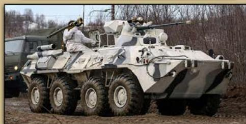
Russian Infantry fighting vehicle, first fielded in 2013 and is the latest version of the BTR-80 APC series. Three man crew, with room for seven fully equipped troops. Main armament is a fully stabilized 30mm auto cannon, laser range finder. Advanced crew protection and armor shielding, 16 tons vehicle weight. Maximum speed, 55 mph top speed. Other variants include the amphibious naval BTR-82AM and up-armored BTR-82AT. In service with Russian ground and naval forces, Kazakhstan and Azerbaijan.
