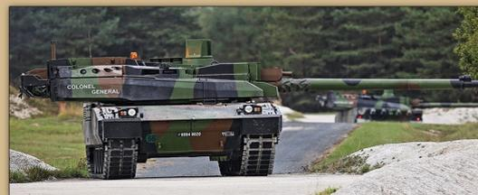
French third-generation MBT, in service since 1992. Three-man crew, weight is up to 57.4 tons. Main armament is an autoloading 120mm gun (NATO round compatible) and 40 round on-board capacity. Secondary armament consists of 12.7mm and 7.62mm machineguns. Advanced fire control and digital communication system. It has modular composite armor, and the SXXI variant has reactive layers. In service with: France, UEA, Jordan.
