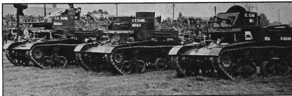
casemates mounting .30-caliber machine guns. It had a 350-horsepower radial air-cooled aircraft engine, and it could do over 26 miles per hour. Its suspension and track parts were the same as those on the new light tank and combat car. It was a success.
