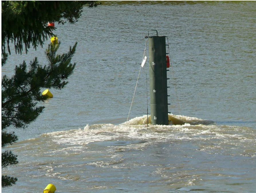
Figure 3. A T-72 tank fully submerged during snorkeling training uses the training snorkel. The crew can exit through this large snorkel, but it is not used in combat. (Photo courtesy Wikimedia)
