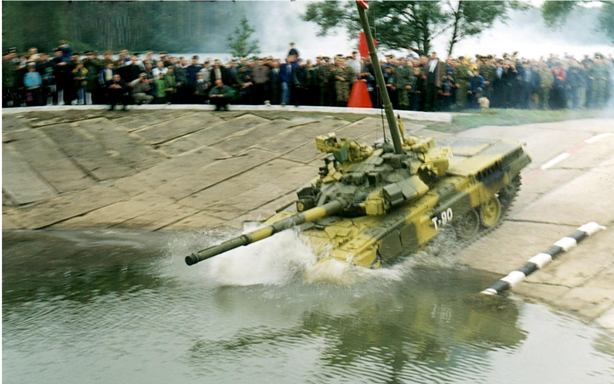
Figure 2. A T-90 tank with its wading snorkel erected enters a concrete pool at a Russian training site. (Photo by Serguei S. Dukachev)
