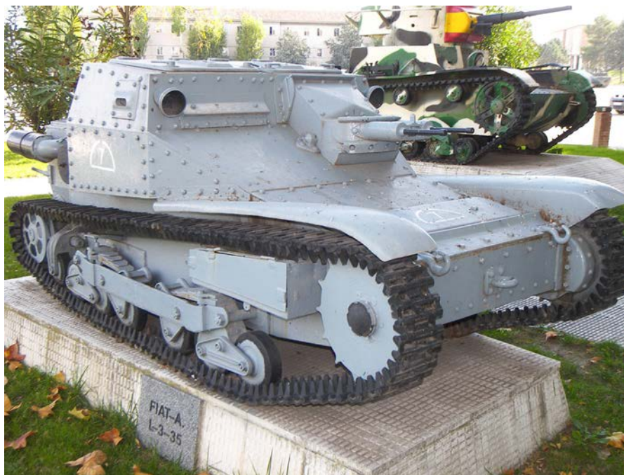
Figure 2. This is the Italian light tank Fiat L-3 CV 35 made by Fiat-Ansaldo. A total of 155 tanks were provided by Fascist Italy to Nationalist Spain. The first L-3 tanks arrived in Spain in late August 1936, the first modern tanks entering service in the Spanish Civil War. Outgunned – they were armed with only two fixed machineguns – they were not a match to Soviet tanks. They did not even have a turret; to aim the machineguns, the whole tank had to move. Some 60 Italian tanks survived the war and even continued in active service until the early 1950s in Spanish cavalry units. (Author's collection)
