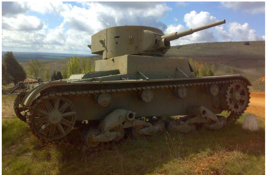
Figure 4. This is a T-26B Soviet light tank furnished by the Soviet Union. Those tanks started to arrive into Republican Spain in October 1936 and were real tanks with a main gun and machineguns. They were heavier than the ones provided by Germany and Italy to Nationalist Spain and better protected. The Soviet Union provided 286 T-26B tanks to the Spanish Popular Army, and more than 130 ended up in the service of the Nationalist Army by the end of the war. They remained in active service until the early 1950s. This picture was taken near a memorial for the civil war on what was once the battlefield of the Ebro, which took place in 1938. (Photo by COL Anthony J. Candil)
