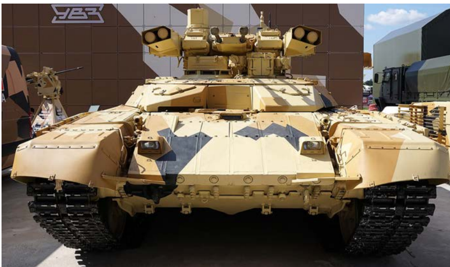
Figure 4. The latest model of BMPT-72 destined for the export market. Note the redesigned turret and lack of forward-facing grenade launchers. (Photo copyright Vitaly Kuzmin. Licensed under a Creative Commons Attribution-NonCommercial-NoDerivatives 4.0 International License.)
