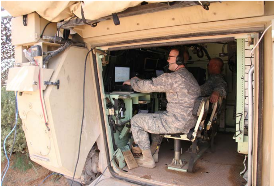
Figure 4. Combined-arms battalion (CAB) mobile tactical CPs are M1068 tracked vehicles with integrated mission-command and radio capabilities, allowing commanders to “command from the hatch.” (U.S. Army photo)
