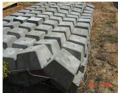
Articulating concrete mats are used to harden low-water crossing sites along tank trails at Fort Benning
