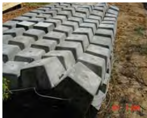
Articulating concrete mats are used to harden low-water crossing sites along tank trails at Fort Benning
