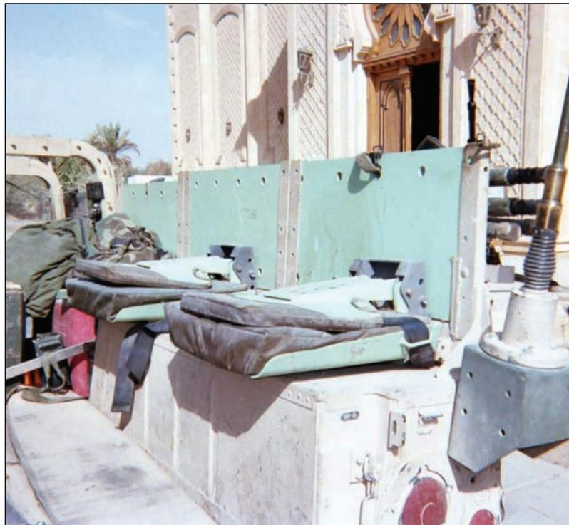
Figure K-11. Closeup of sections of Bradley fighting vehicle spall liner armor applied to exterior of cargo bed.
