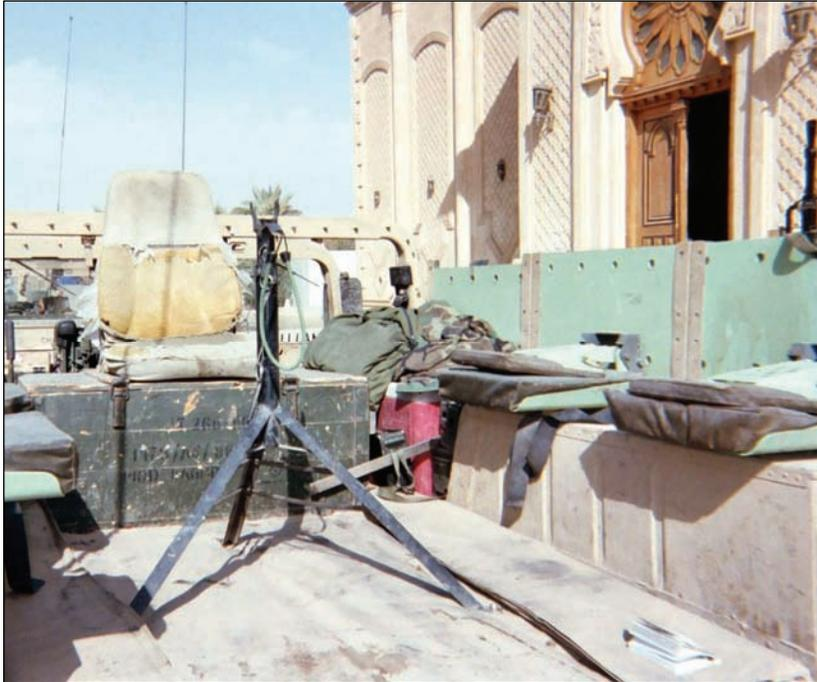
Figure K-10. Unit-produced tripod and modified armor.
