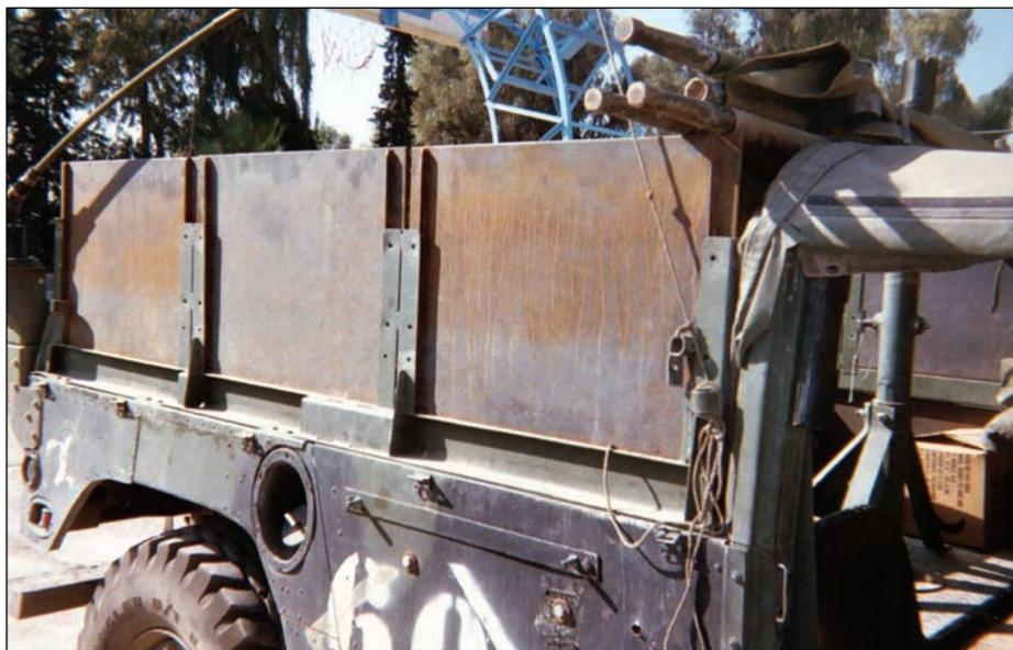
Figure K-12. Unit-installed steel armor.
