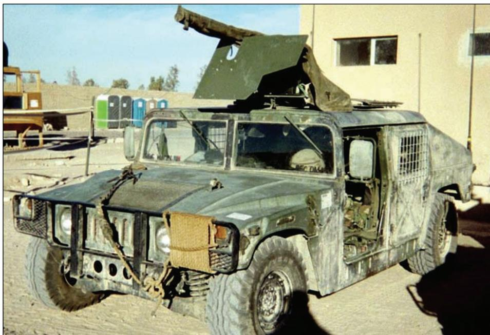
Figure K-1B. Army-issue, roof-mounted, gun-ring armor.
