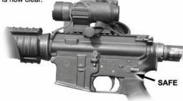
2. Attempt to place the selector lever on SAFE. If the selector lever cannot be placed on SAFE because the weapon is not cocked, proceed to Step 3.
