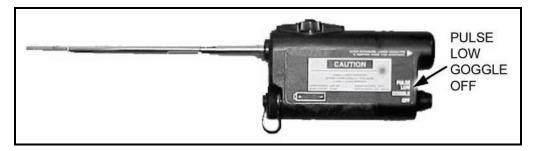
Figure 2-47. Borelight with a 5.56-millimeter mandrel.
