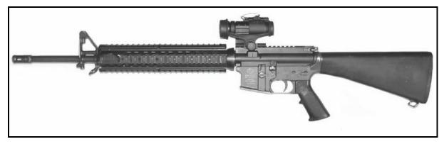
Figure 2-23. Mounting the M68 on an M16A4 rifle or M4-series carbine.
