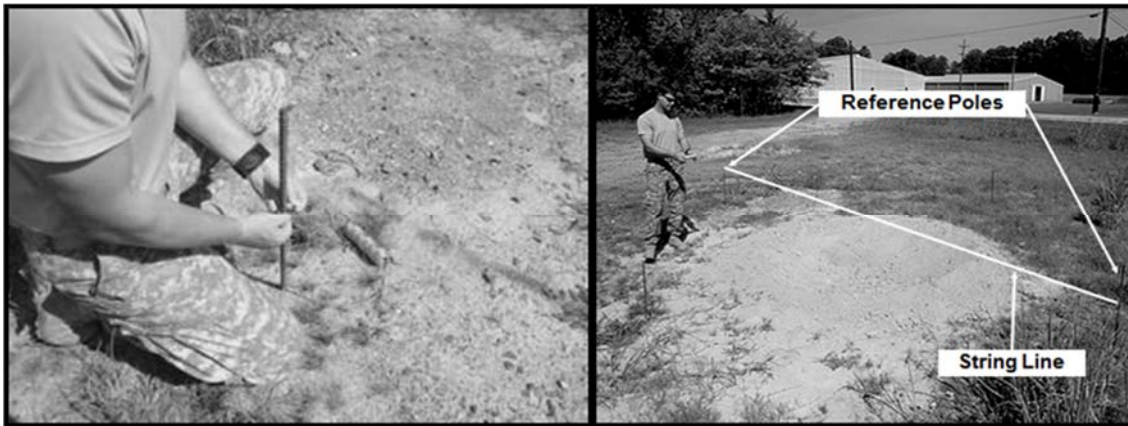
Figure G-9. Step 2. Establish reference data points
