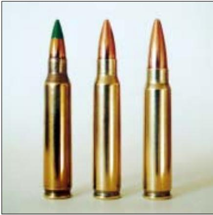
**Figure 1** — Low cost options for improving performance over the 5.56x45mm round (left), are the 6x45mm (center), and 6.5x42mm MPC (right). These cartridges are compatible with 5.56mm magazines and bolts, M27 metallic links, and the M249 feed mechanism.
