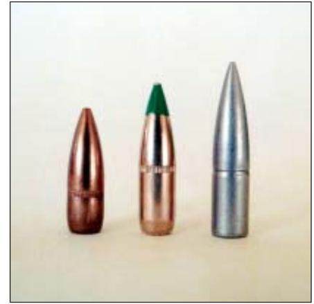
**Figure 3** — 5.56mm projectiles: (l. to r.) 55-grain M193 Ball, 62-grain M855 Ball, 77-grain “heavy ball.” The steel jacket of the heavy ball bullet is tougher than the gilding metal jackets of the other two, enabling better penetration of typical battlefield obstacles.
