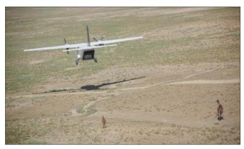
Due to low altitude of the aerial delivery platform, the resupply bundle descends to the drop zone within seconds; this short descent time limits the ability of the enemy to observe the bundle.
