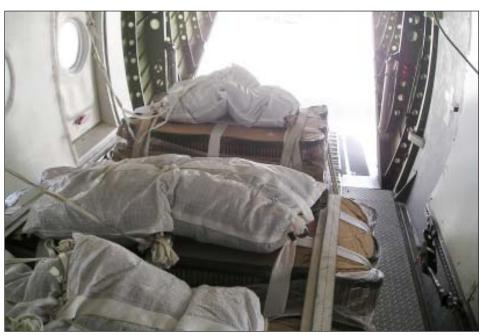
Bundles of fully rigged 105mm ammunition are prepared to be dropped from a CASA 212 aircraft. The bundles are configured to allow a two-man team to lift them into the back of a trailer or variants of the HMMWV.
