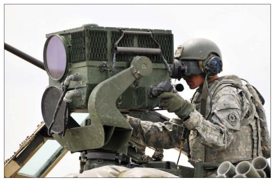
A Soldier with the 4th Squadron, 2nd Cavalry Regiment scans the terrain using a Ground/Vehicle Laser Locator Designator during an exercise at the Grafenwoehr Training Area in Germany on 31 May 2012.
