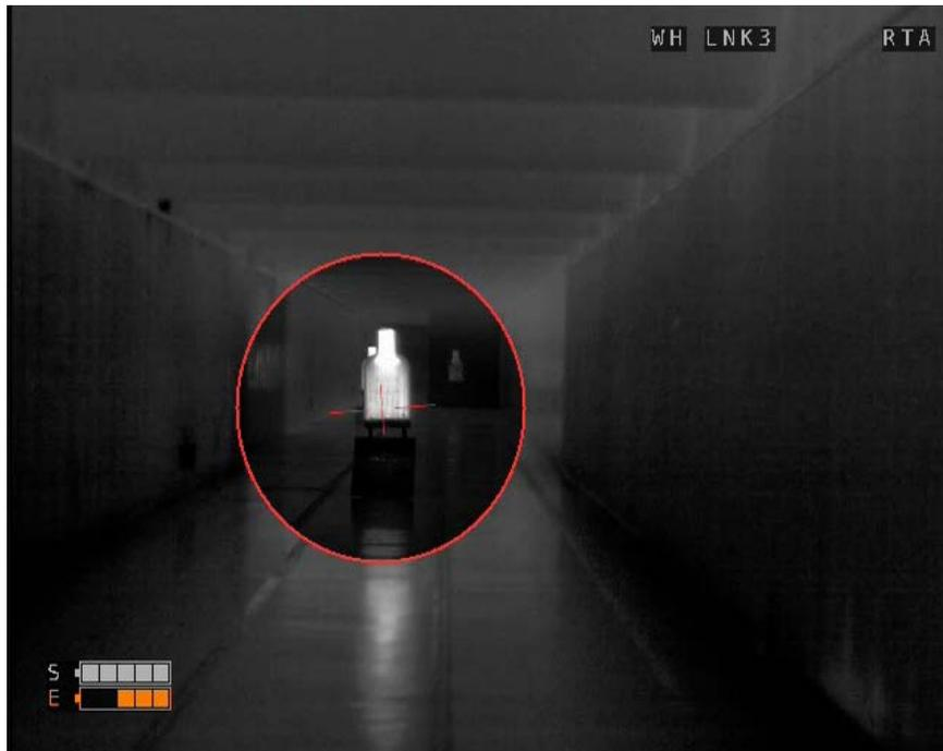
**A shooter fires on a target using an ENVG III on his helmet and a FWS-I on an M4 rifle. (Photos courtesy of PEO Soldier)**
