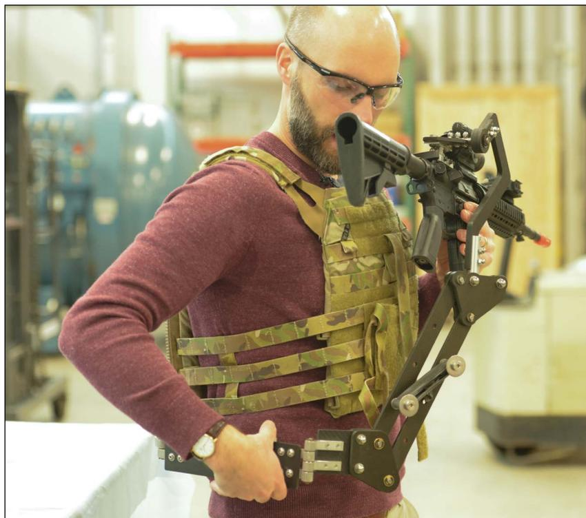
**Army Research Lab engineer Dan Baechle demonstrates how to strap on a mechanical device designed to improve Soldiers' accuracy and reduce fatigue.
