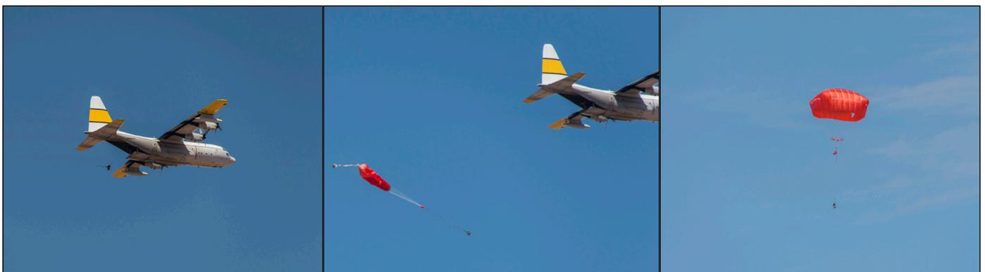
**This series of photos shows a simulated towed jumper scenario with a mannequin that is towed behind an aircraft. The Towed Jumper Recovery System includes an emergency parachute that is released once the jumpmaster cuts the aircraft anchor line cable. (U.S. Army photos)**
