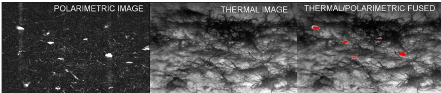
*The images above are examples of identification of hidden booby traps and tripwires using conventional and polarimetric thermal cameras.*
