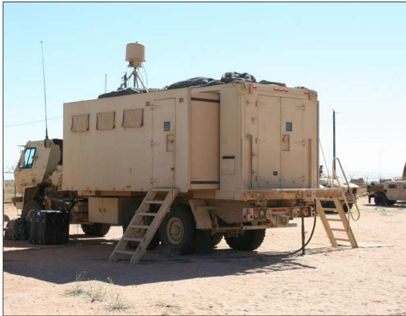
**A tactical command post based on a Light Medium Tactical Vehicle with expandable van is pictured at Fort Bliss, TX, during Network Integration Evaluation 14.1. (U.S. Army photo)**
