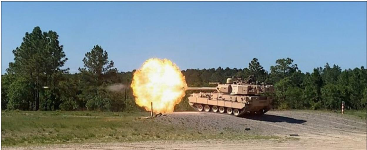
**The Mobile Protected Firepower brings necessary firepower to the infantry brigade combat team's fight. The 105mm cannon, the coaxial 7.62mm machine gun, and the externally mounted .50 caliber machine are the primary armaments for the MPF. (U.S. Army photo)**
