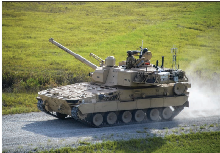
Equipped with a 105mm gun, the M10 will be fielded to light infantry forces and be able to press the attack, disrupting the enemy's intentions while still providing the speed and agility that have been the hallmark of light infantry. (U.S. Army photo)
