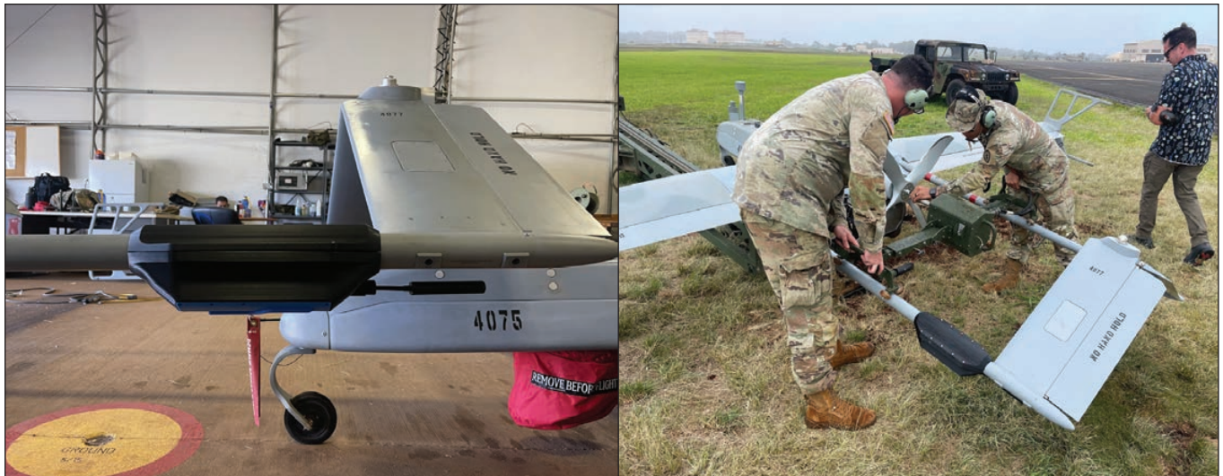
25th Infantry Division Soldiers test mount the Shadow Echo, a partnered project with the 225th Brigade Support Battalion's Allied Trades Shop. The Shadow Echo hopes to expand infantry brigade combat team command and control bubbles through vertical relays.
