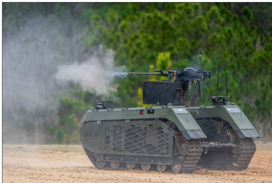
The Milrem THeMIS, a Dutch and German ground-based system combining an unmanned ground vehicle and a remote-controlled weapon station, participates in the 2024 AEWE on 29 January.
