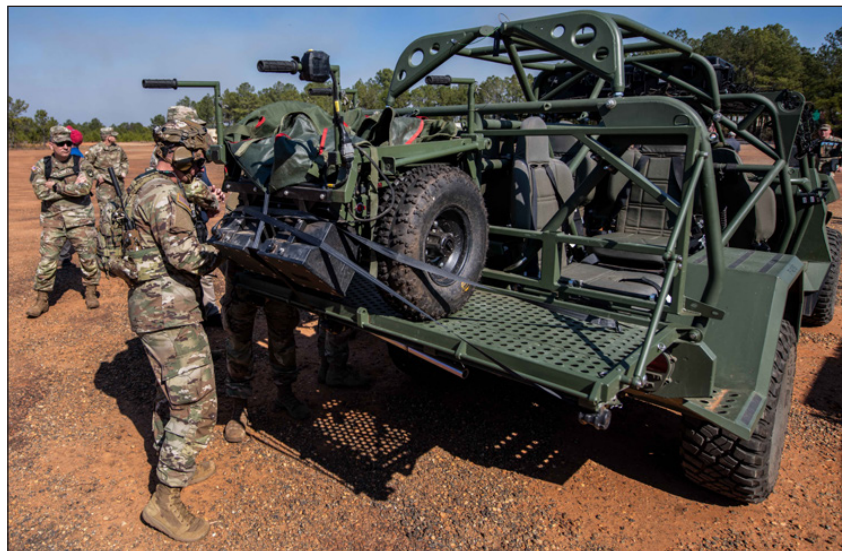
Technology and industry leaders unload and set-up their concepts to demonstrate their submissions on 2 February 2024 at Fort Moore, GA. The Silent Tactical Energy Enhanced Dismount is an all-terrain, electric payload mobility platform which is tactically silent and has zero emissions. (Photos by Patrick A. Albright)
